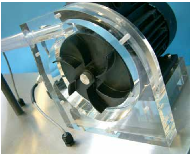
Detail of the Centrifugal Pump (shown with cover removed prior to exchanging the impellor)
