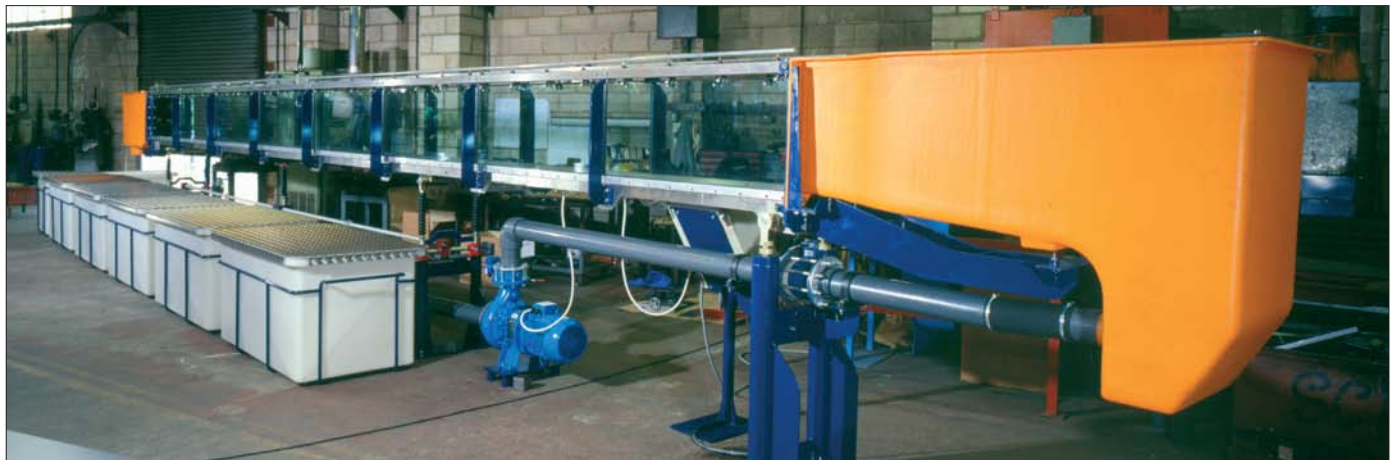
10m working section. The end tanks actually extend the effective length of the flow channel beyond this. S6 MkII Glass sided Tilting Flume
