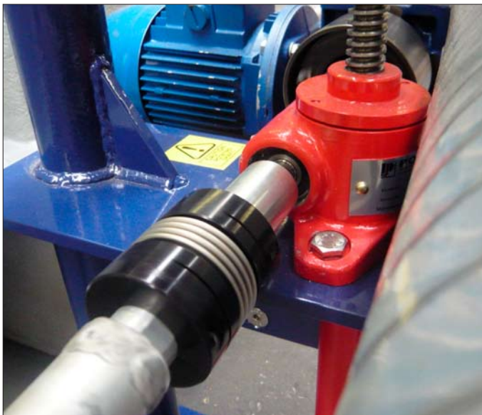
Gearboxes at each jacking point ensures accuracy of the tilting channel bed and the benefits of ease of operation.
