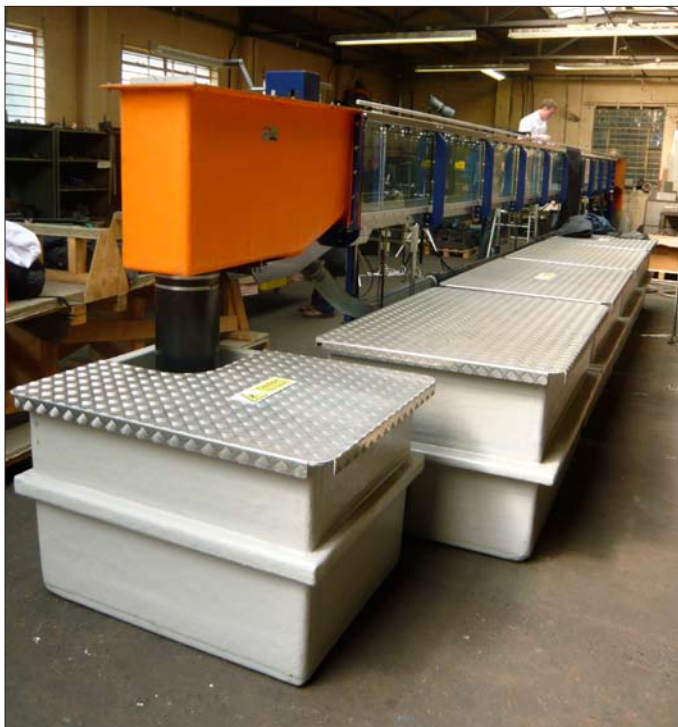
S6MkII view from outflow end showing sump tank arrangement
