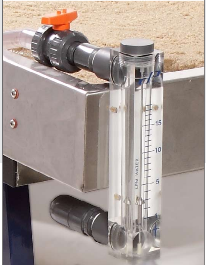
Adjustable flow valve and flow meter
