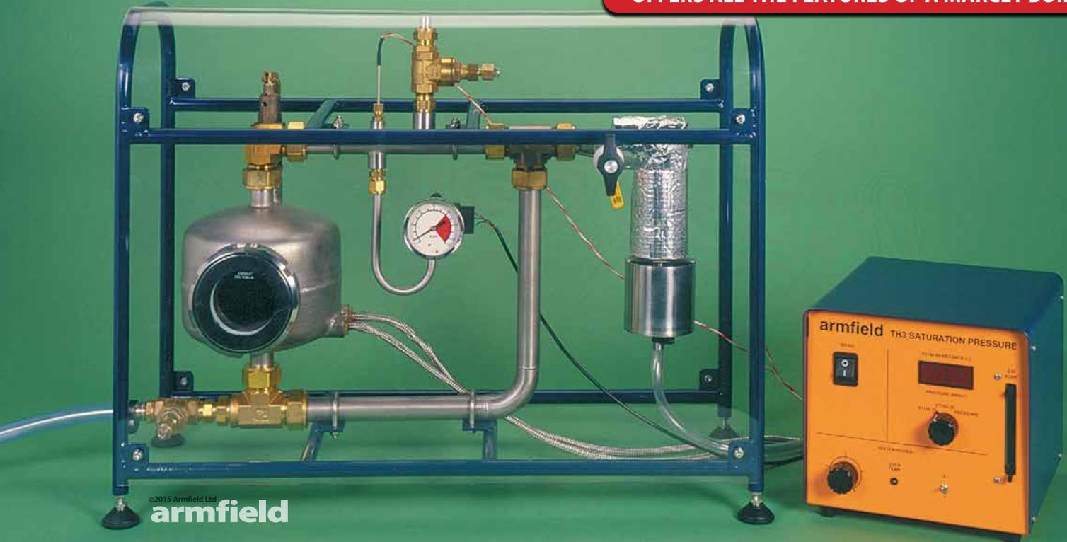
The Armfield Saturation Pressure Apparatus has been designed to introduce students to how the temperature of water behaves at its boiling point with variation in the absolute pressure.
