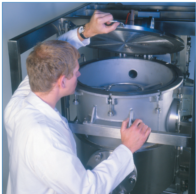
Inspecting the interior of the extractor vessel
