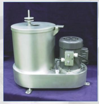
manually rotated into the spinning liquid which thereby is drained from the bowl. The first material discharged will be the purified light phase. After this the heavier phase (if liquid) can be drained in the same fashion by continuing the rotation of the tube. Alternatively, with more viscous materials and solids, the machine is stopped and the bowl quickly removed for cleaning.
