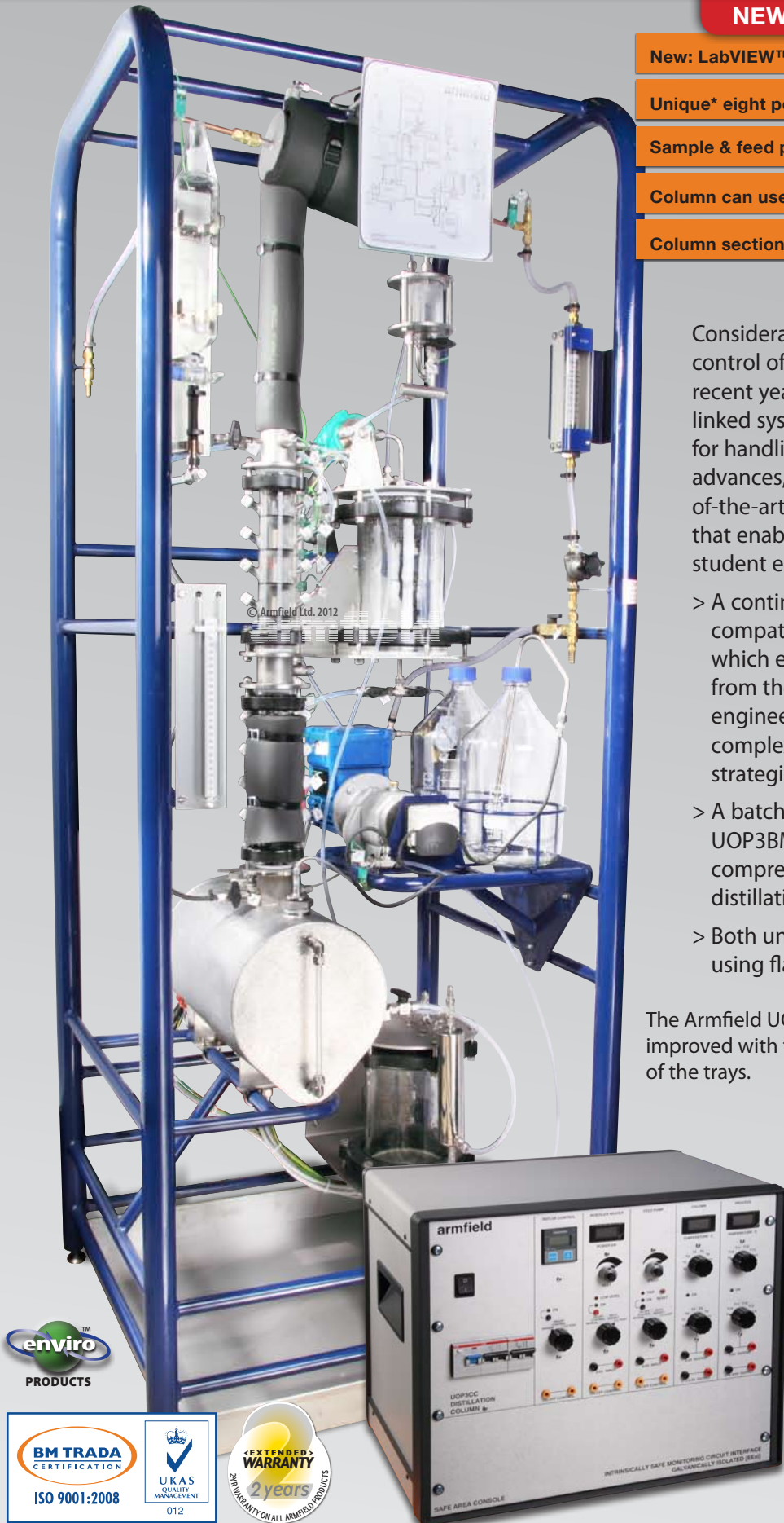
Above: Computer interfaced distillation column UOP3CC shown with safe area console
