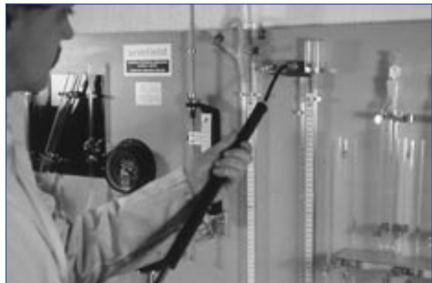
Pressurising a manometer
