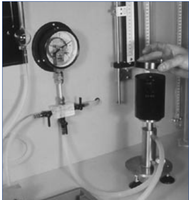
Calibration of a Bourdon gauge using a dead weight calibrator
