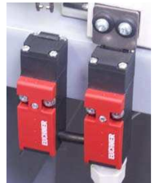
Two interlocked safety switches that cut motor power if the hoods are lifted during operation
