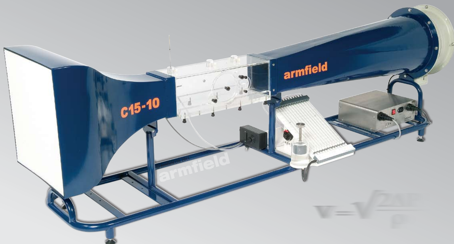
C15-10 shown with the C15-11 Inclined Manometer Bank Accessory fitted
