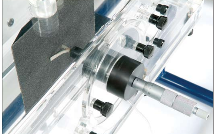
Pressure distribution around one side of cylinder (C15-23) - Tapping 1 upstream.
