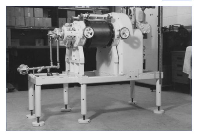
The Armfield Drum Drier consists of a nip fed twin cylinder drying machine, cast from Meehanite GA, cast-iron with combined endplates and trunnions. The rolls are accurately ground on the circumference, bored internally to ensure even heat transference, and suitable for working with steam at up to 5.5 bar. The rolls are carried in grease lubricated bearings which are housed in circular endplates mounted on the base plate of the machine.
