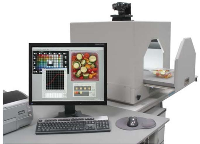
The system has the versatility to measure objects as small as a grain of wheat and with a total field of view of around 40 cm x 50 cm, it can accommodate a wide array of food types.
