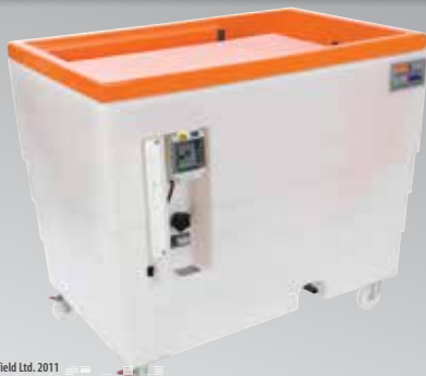
F1-10 Basic Hydraulics Bench
