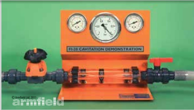
F1-28 Cavitation Demonstration
