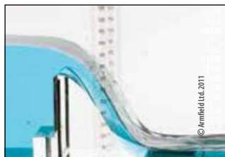
Smooth flow over an Ogee Weir.
