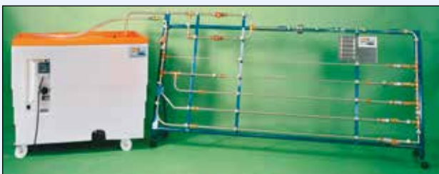
NEW F1-33 Pitot Tube Demonstrator
