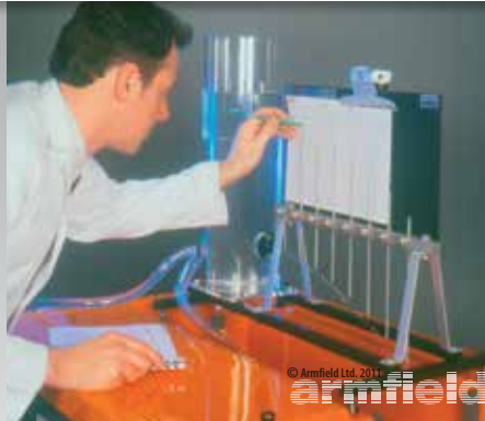
F1-17 Orifice and Free Jet Flow
