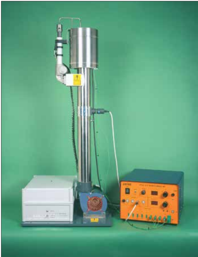
Computer Controlled Radiation Errors in Temperature Measurement - HT16C
