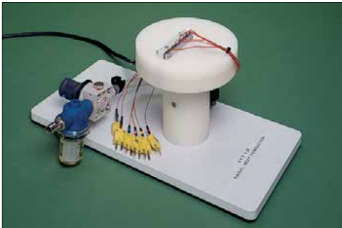
Computer Controlled Radial Heat Conduction - HT12C
