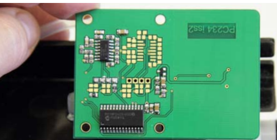
Cartridge microcontroller containing sensor calibration
