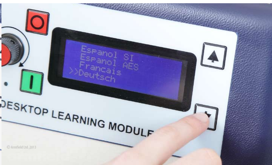
Multiple language support and SI or American Engineering Systems units display options
