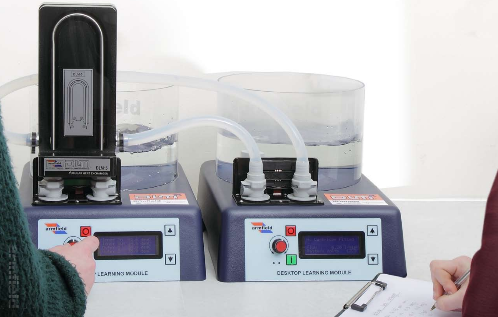
Students run a series of experiments on a pair of DLMX base units fitted with the DLM-5 Tubular Heat Exchanger cartridge. One unit controls the inner tube flow and the other controls the outer tube flow.
