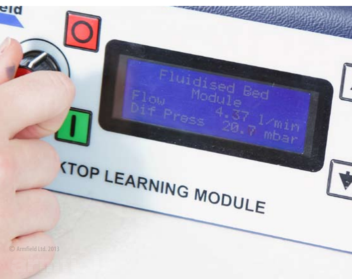
Simple pump speed control and flow rate display
