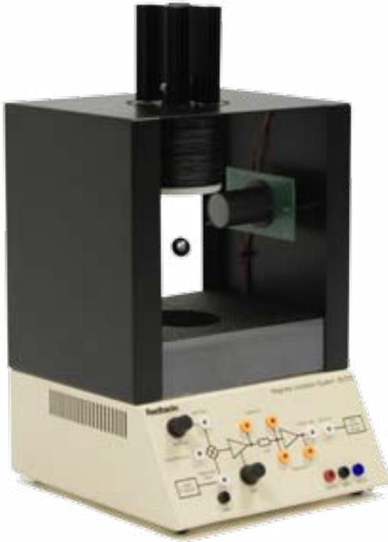
This classic magnetic levitation control problem is now presented in a new and innovative form. A 25 mm diameter, hollow steel sphere is suspended in space with visually appealing results and convenient time constants.
