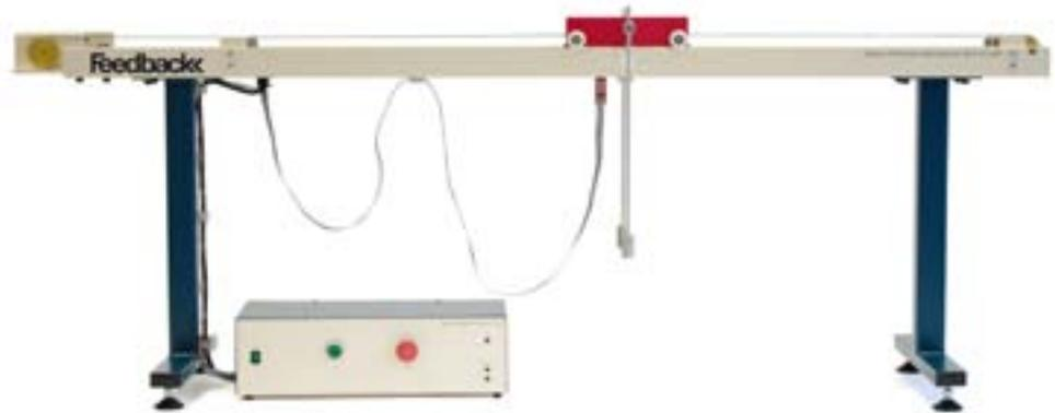
The Digital Pendulum is a modern version of a classical control problem; that of erecting and balancing a free swinging pendulum in its inverted position or moving a hanging pendulum in a controlled manner.
