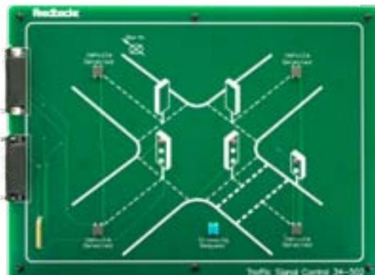
The traffic light system's simple sequence application allows control of a crossroads to be implemented on a time sequence basis. The control program can be further developed to cope with interrupts generated from pedestrian crossing requests or off-peak vehicle detector inputs.
