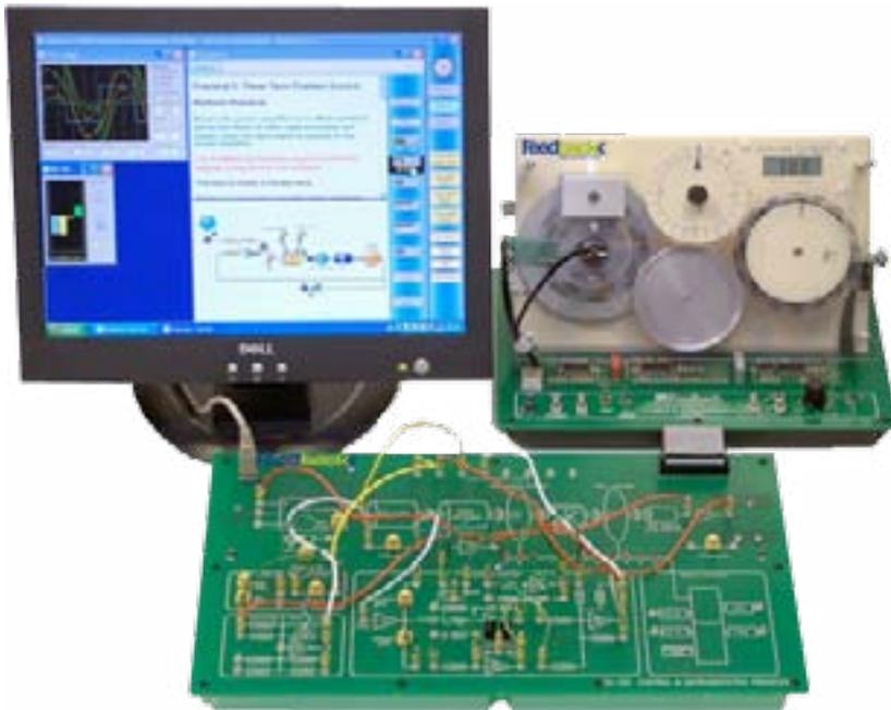
This trainer allows the investigation of control system principles by using a servo mechanism comprising a d.c. motor, a variety of sensors and both analogue and digital controllers. Students are also introduced to the fundamentals of transducers and signal processing.
