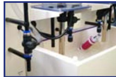
The Coupled Tanks set-up is a model of a chemical plant fragment. Often tanks are coupled through pipes and the reactant level and flow has to be controlled. The Coupled Tanks experiment is designed so that the system can be configured.
