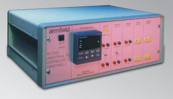
The unit consists of a Honeywell UDC3200 PID controller mounted in a standard console along with connectors for inputs and outputs to selected instructional equipment from the Armfield range. In addition to the analogue input/output, relay and alarm sockets are provided for a digital output control action. An RS232 port enables serial communications with a user provided PC.
