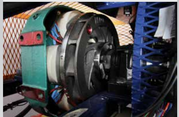
Integrated eddy current dynamometer to vary engine load
